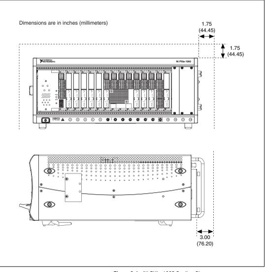
Figure 2-1. NI PXIe-1065 Cooling Clearances
